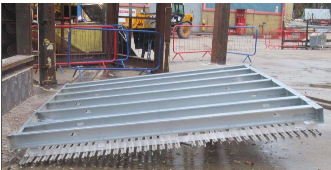
SUPPORT FRAME REMOVED FROM TEST RIG
