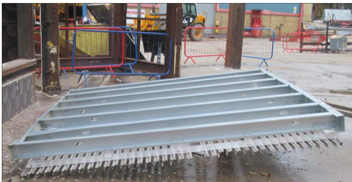
SUPPORT FRAME REMOVED FROM TEST RIG
